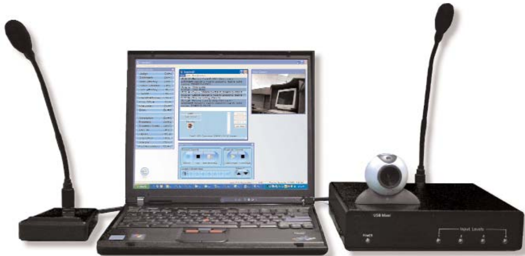
Illustrates Encompass as a portable solution using VIQ-4 (USB mixer) and Logitech QuickCam Pro 3000 digital camera
